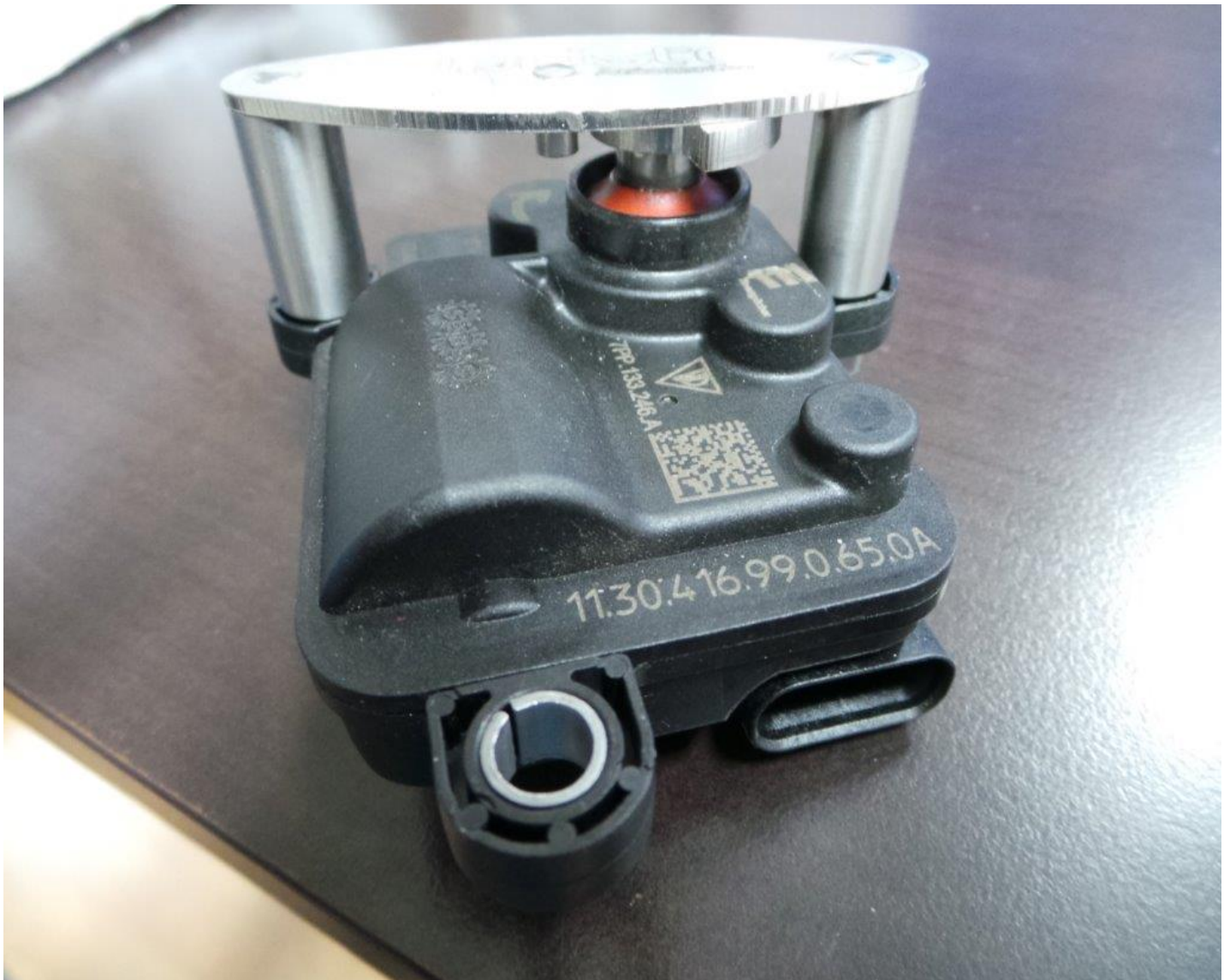
Abb.39-44 Anschlagplatte E-Motor pic. 39-44: stop plate E-motors
