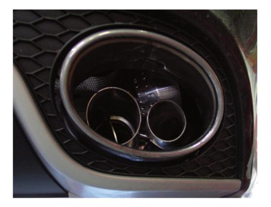
Regarding the heat elongation, the whole system shuld be aligned/fixed as far as possible to the front. This prevents the system to strike against the vehicle while expanding.
