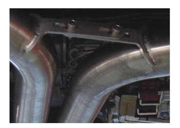
If all connections are tightened, it is recommended to make a visual control check. For further inspection, the system can be manually moved back and forth several times, in order to determine possible contact with other vehicle parts. If necessary, adjust the alignment of the system until it rests correctly everywhere.
