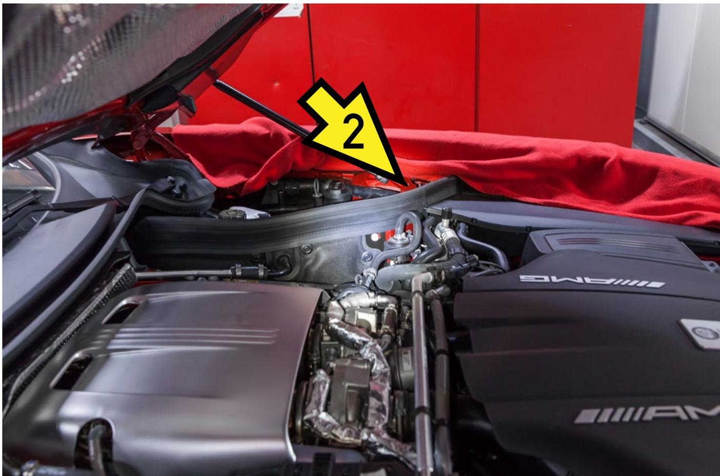
2. Antenne (langes Kabel)/antenna (long cable)
