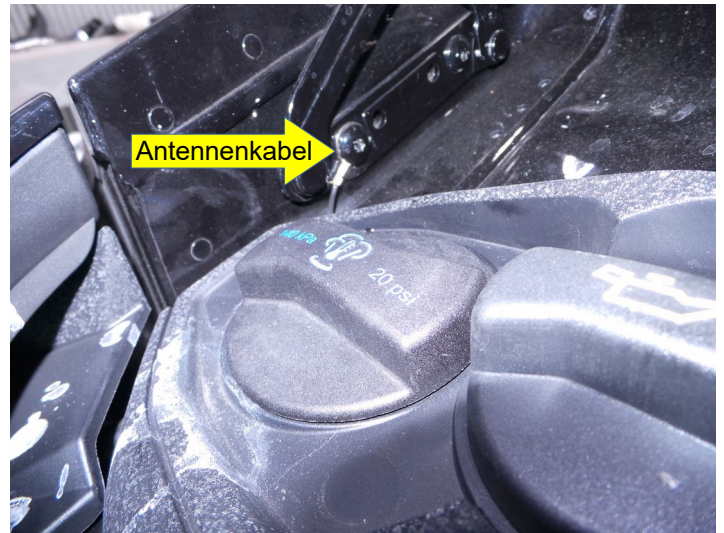
Abb.21: Position Antennenkabel Pic. 21: Position antenna cable
