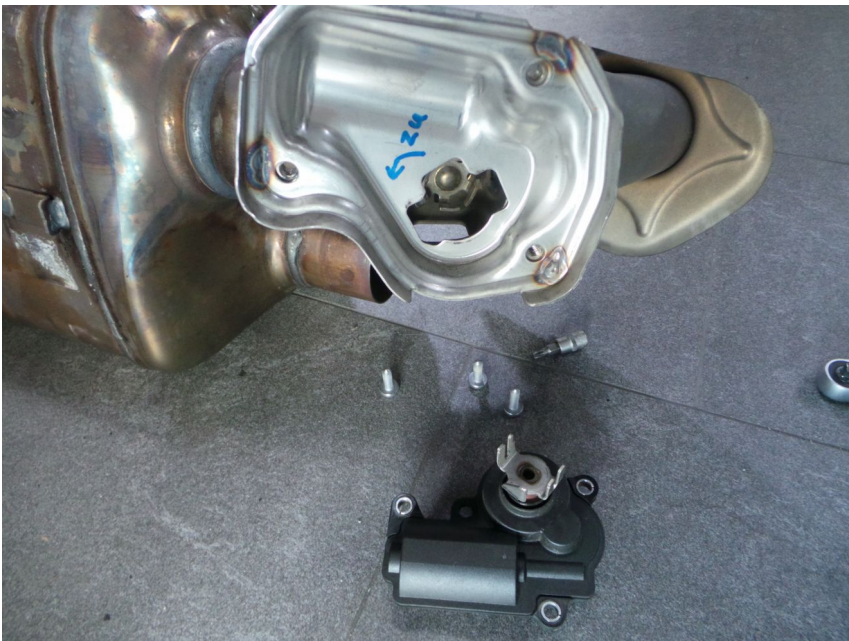
Abb. 13-14: Demontage der OEM Aktuatoren Pic. 13-14: Disassembly of the OEM actuators
